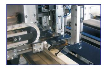
At the mounting station, the mounting head takes up in one operation all the clips that are required for the element to be machined. At the same time the frame is fed in via felt-covered belts and clamped. The mounting head is positioned at the respective frame piece and sets the clips. The number of clips to be attached at the same time depends on the number of setting units that thus define the machining time.
