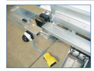
It is possible to use a cutting-to-length tool in order to punch and cut all fittings components to be cut to length for mounting on to the drive and top sides of the sash. The elongated fittings are cut-to-length and at the same time embossed with a new connection hole.
